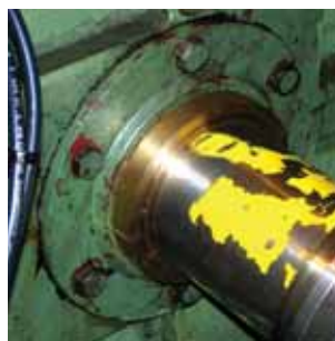
100mm LabTecta-RDS™ installed on a gearbox (Case Ref: 3370)
